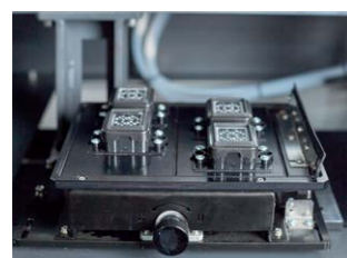
Station de nettoyage
