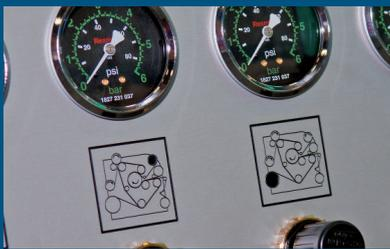
8. Air pressure operated paper tension setting
